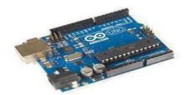
The Arduino board is a microcontroller development platform that will be central When making something you will be building the circuits and interfaces for interaction, and telling the microcontrollerhow to interface with other component
